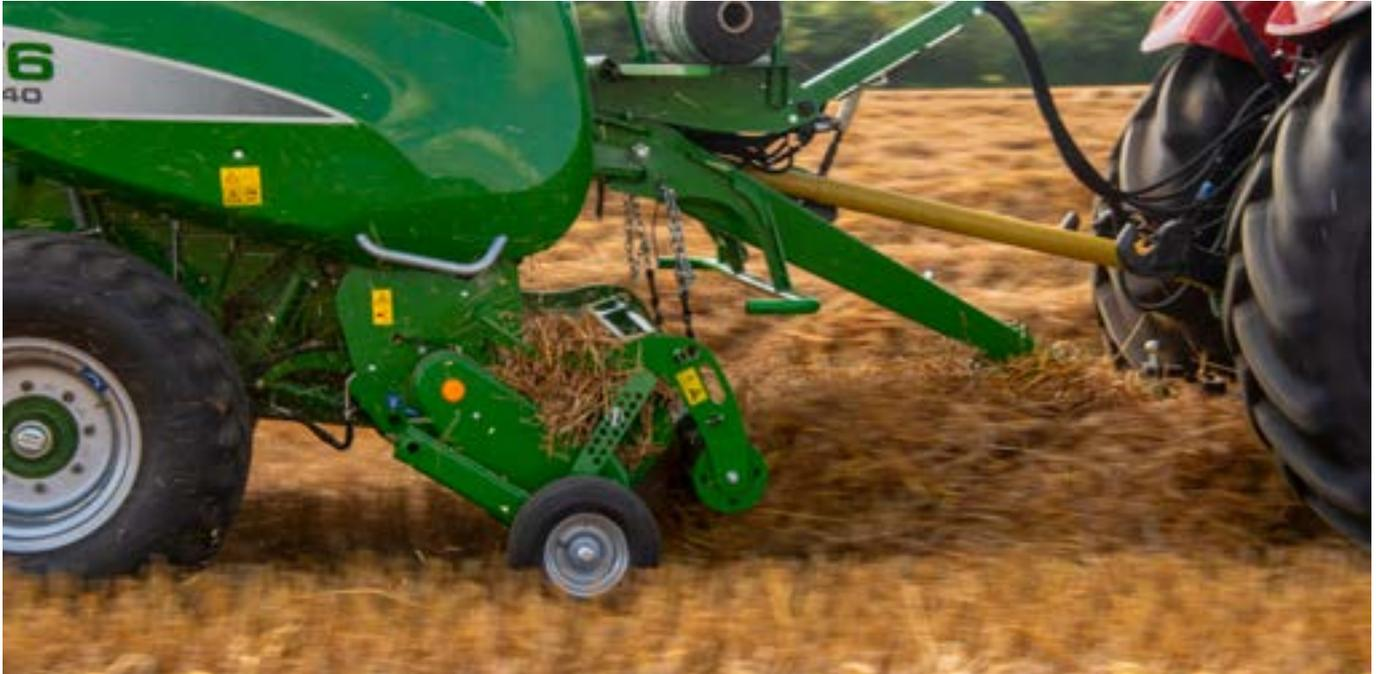
The new tapered feed channel encourages the crop to flow from the pick-up and then move towards the rotor and into the bale chamber, maximising throughput. McHale have also moved the lateral feed augers forward and their ends are angled towards the rotor for improved crop flow.
