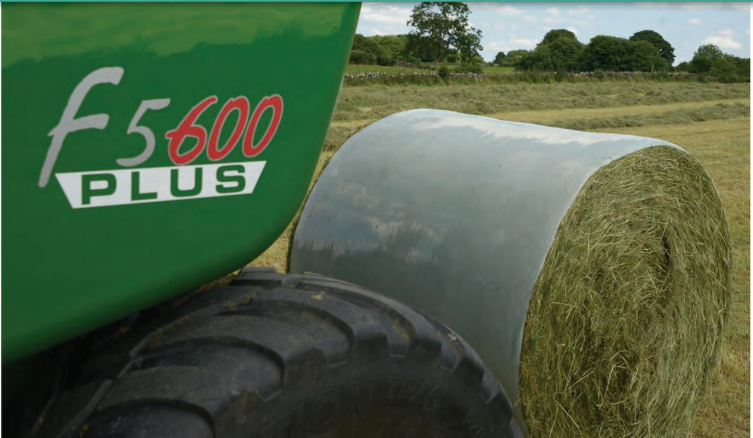
Film on film technology refers to the application of film to the barrel of the bale in the bale chamber. The film binds the bale together which eliminates the need for string or net wrap. The film that binds the bale together forms a wrap layer and gives better film or plastic coverage on the largest surface of the bale.
