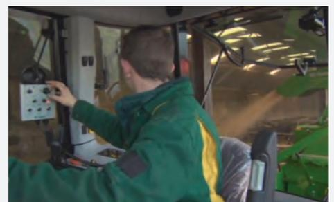
The chute is joystick controlled, allowing the operator to adjust the chute height and the shoot direction easily from the control console in the tractor cab. The chute can be rotated 300°, which allows material to be spread on the left, right and behind the machine. The chute may also be lowered to blow material on to the feeding slide for better control when distributing feed along a barrier.
