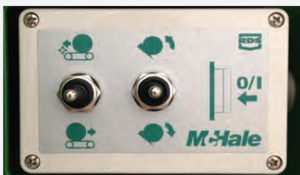
An external loading control comes fitted as standard which will allow for the conveyor floor and the tailgate to be operated when removing the netting or wrap whilst loading a bale. The tailgate and conveyor alignment on the machine body take the largest size square bales without the need for extensions to the tailgate.
