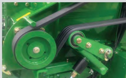
The McHale C4 Silage Feeder & Straw Blower range of machines are designed to allow the rotor work independently from the flywheel. This allows the flywheel to be at full RPM before any fodder material is fed into the rotor.
