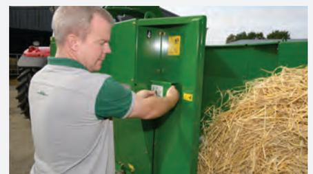
To prevent accidental operation of the controls, a safety button on the side of the External Loading Control must be pressed while operating loading functions at the rear of the machine.
