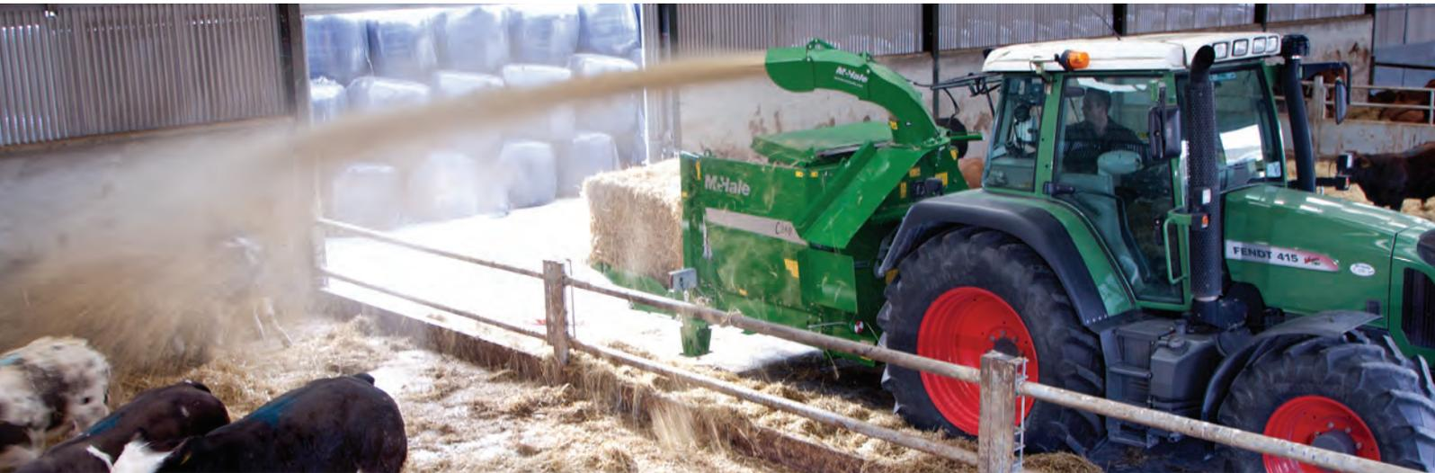
The McHale C4 Silage Feeder & Straw Blower Range is fitted with a three-stage chute. This three-stage design minimises resistance and allows for maximum blow distances to be achieved, especially when blowing straw in confined spaces.
