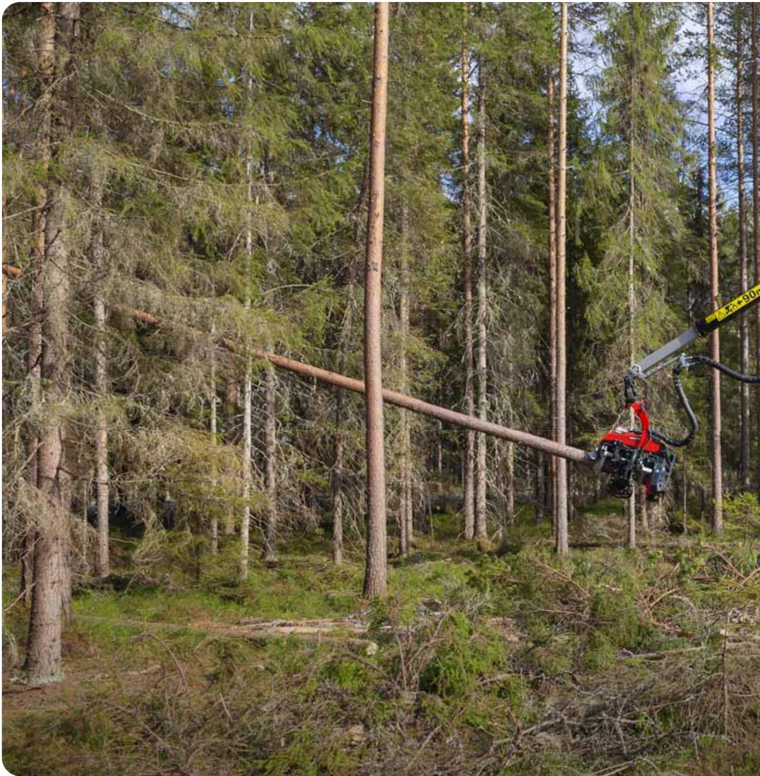
The modern harvester has its origins in models that were designed back in the early 1980s. The 901 was launched in 1984, and at the time it was the world's first single-grapple harvester with a specially designed harvester chassis. Up until then, a modified forwarder chassis was often used. The 901 also saw the introduction of the stable Komatsu concept, which remains essentially the same today.
