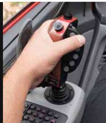
**New!** EME joysticks with sequence control. Ergonomic and adjustable hand controls that allow the operator to customise most button functions.
