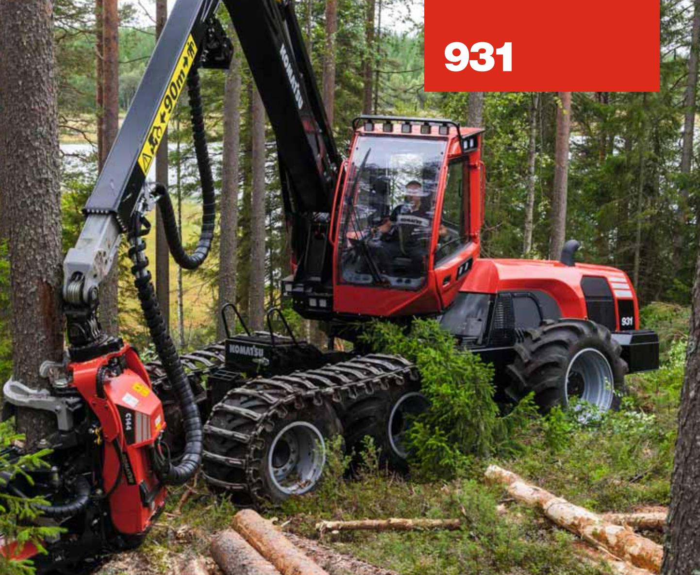
the lifting power you need. What's more, the smart pressure and flow optimisation means that you can do several things at once, such as slew and feed, with full hydraulic power and maintain a considerably higher work rate. To this we can add a full 360 degrees of cab rotation that enables you to process more from the same spot, which optimises forwarding.
