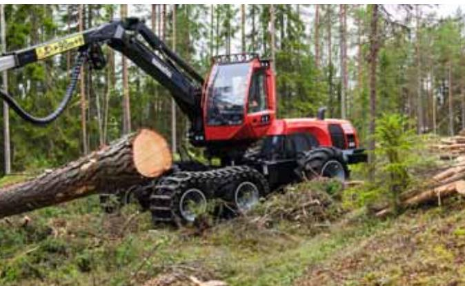
The unique 3-pump hydraulic system means that you can operate several functions simultaneously, such as slewing the crane and feeding a log while manoeuvring the machine, without losing hydraulic power.
