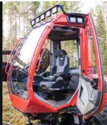
New large and noise-reducing cab with larger windows that provide superior visibility upwards, downwards and to the rear.
