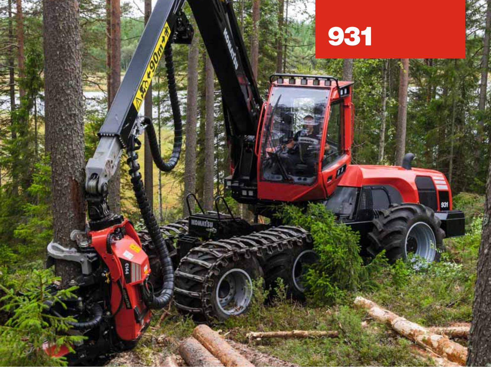
the lifting power you need. What's more, the smart pressure and flow optimisation means that you can do several things at once, such as slew and feed, with full hydraulic power and maintain a considerably higher work rate. To this we can add a full 360 degrees of cab rotation that enables you to process more from the same spot, which optimises forwarding.
