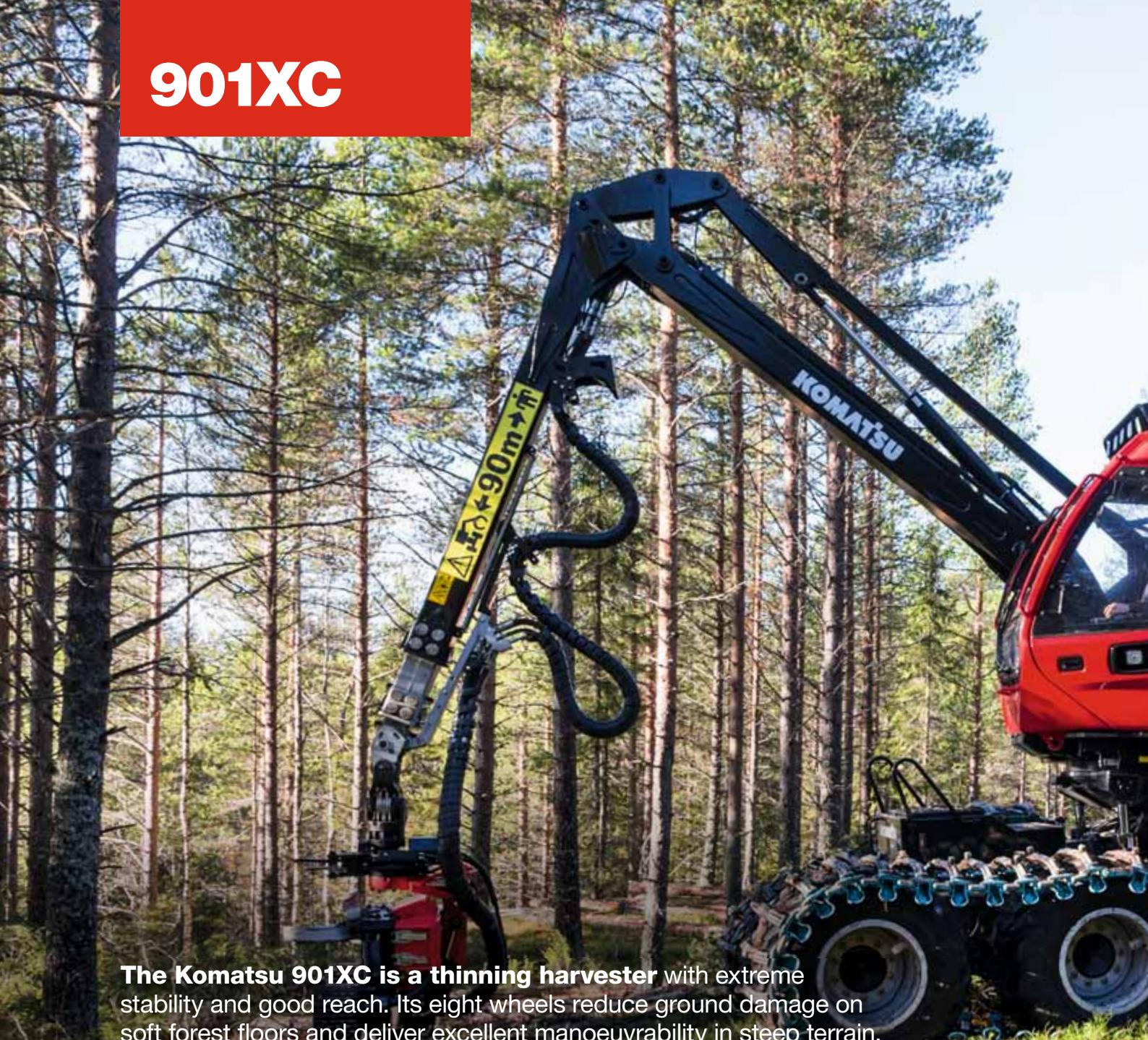
**The Komatsu 901XC is a thinning harvester** with extreme stability and good reach. Its eight wheels reduce ground damage on soft forest floors and deliver excellent manoeuvrability in steep terrain.
