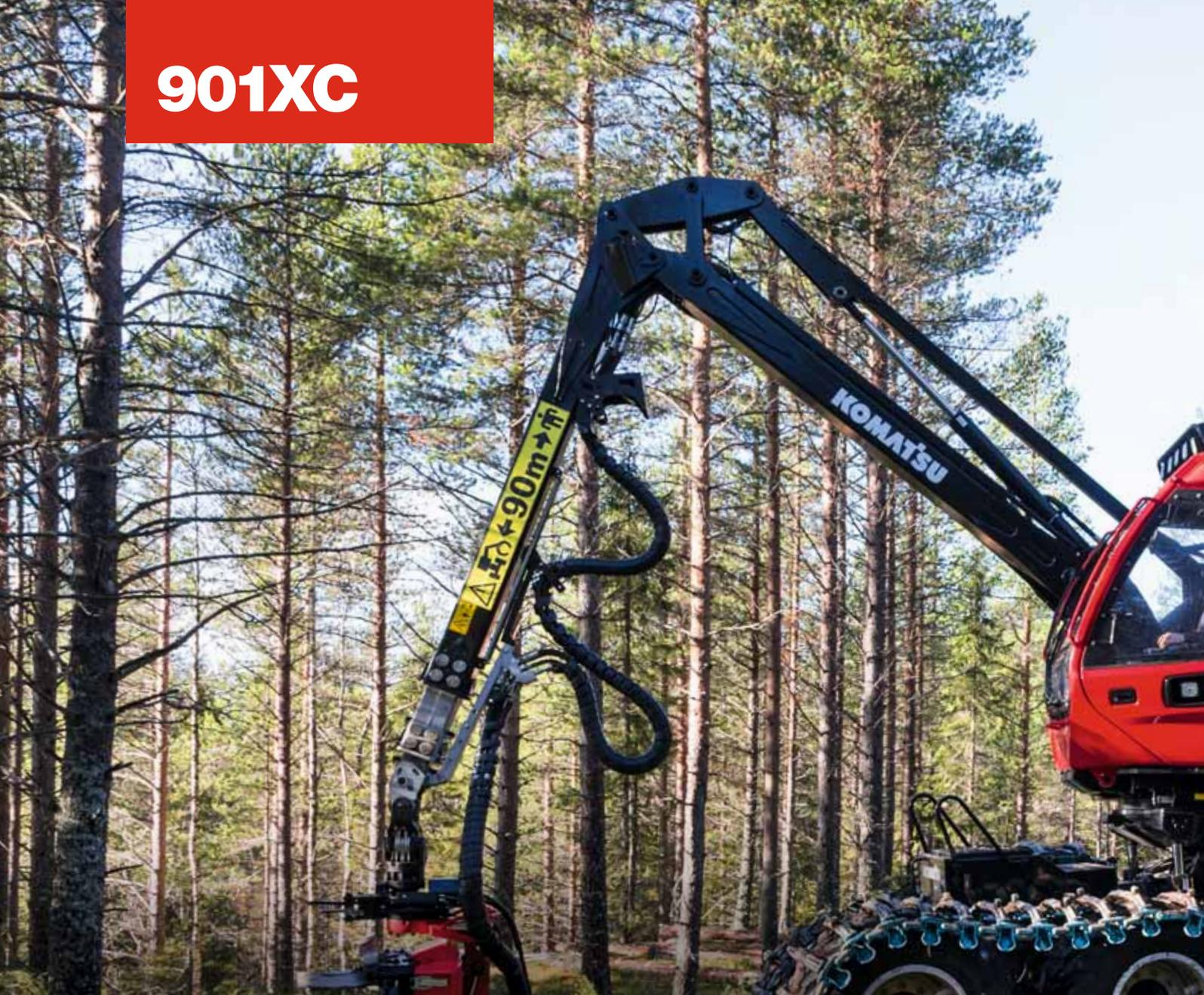
**The Komatsu 901XC is a thinning harvester** with extreme stability and good reach. Its eight wheels reduce ground damage on soft forest floors and deliver excellent manoeuvrability in steep terrain.
