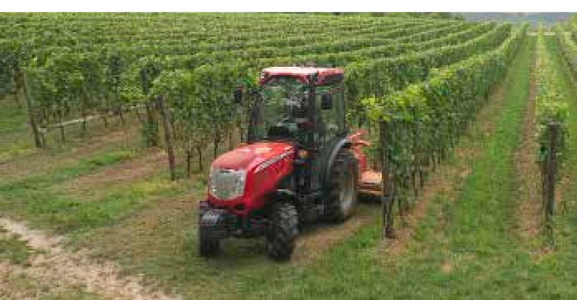
The X4V is McCormick's new specialty vineyard tractor. All five models in the range are powered by the new Deutz TCD L4 2.9L, 4-cylinder engines that cover maximum power outputs from 70 to 102 hp at 2200 rpm. All engines meet Stage 3B / Tier 4 Interim emissions standards and are equipped with exhaust gas recirculation system (EGR), diesel oxidation catalyst (DOC) and Engine Memo Switch to store engine rpm. These tractors feature a 80L fuel tank for extended run-times without refuelling.
