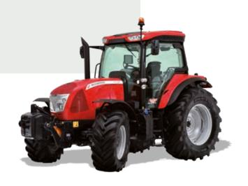
McCormick X6.4 is available in 3 models featuring 121 HP, 133 HP and 140 HP power ratings, 4-cylinder 4,500 cc Betapower Fuel Efficiency emissionized STAGE 4 / TIER 4 FINAL engines with SCR + DOC exhaust gas aftertreatment system and with a VT-Drive 3-stage continuously variable transmission manufactured by Agro Tractors.
